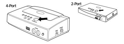
You can directly select a connected computer by pressing the Selector Button on the switch. The LED will be lit above the number to indicate which port is currently selected.
